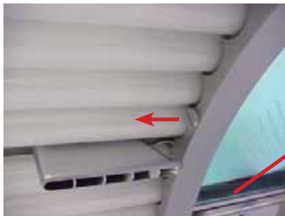
Illustr. 5-8 Dismantling the tube cover
