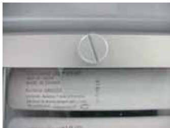
Illustr. 5-4 Loosen screws
