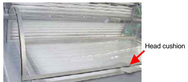
Fig. 5.2 Opening the acrylic pane seals
