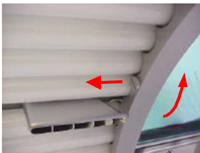
Fig. 5.6 Dismantling the tube covering
