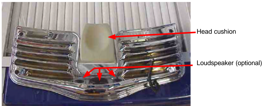
Fig. 4.2 megaFlex – Head cushion and loudspeaker
