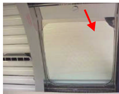
Fig. 5.7 Removing the filter pane frame
