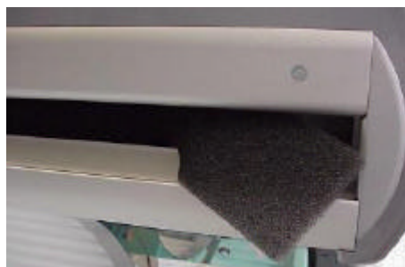
Fig. 5.12 Replacing the filter mat
