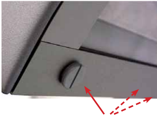
Illustr. 5-2 Release the four screws of the canopy pane
