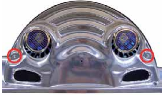
Illustr. 5-6-2: Undo the screws holding the chrome covering
