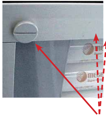
Illustr. 5-3 Release the four screws of the lateral pane
