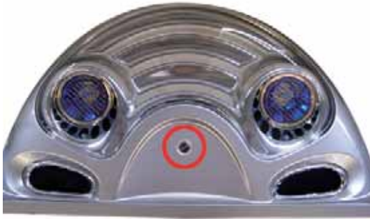
Illustr. 5-6-1: Undo the screw holding the outer covering
