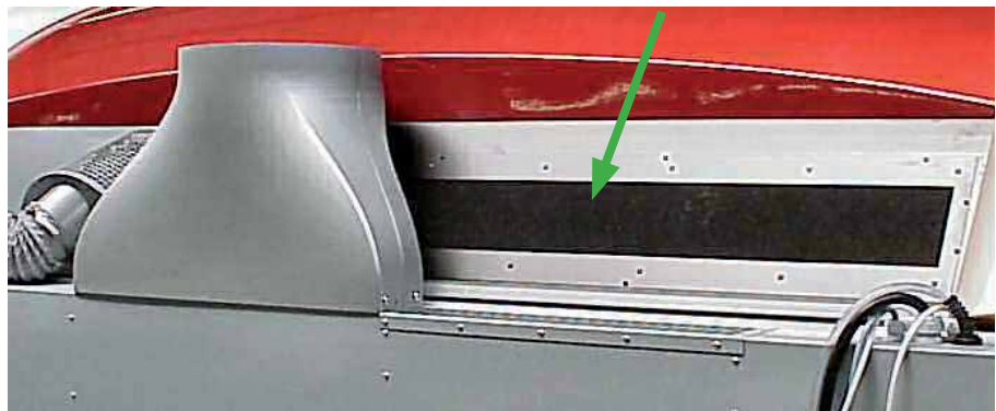
Illustr. 5-16 Replacing the filter mat
