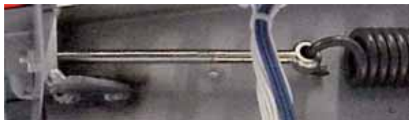
Figure 3-15 Spring compressor The spring has to be secured against torsion while tensioning and relaxing.
